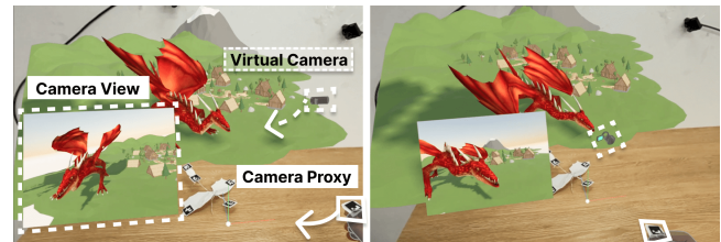
Figure 10: Previs example. A user prototypes a scene where a dragon lowers its wings and head. The animation is made by keyframe in advance, and the user moves a wooden block while playing the animation, which is the physical proxy of the camera. The virtual dragon and the captured scene by the camera are visualized in the real environment.
