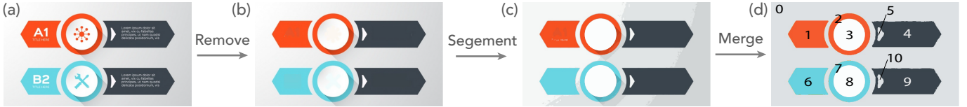
Fig. 3. Three steps to identify artistic elements in an infographic: removing graphical data elements, performing color segmentation, and merging segments with similar hues.
